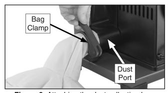
Figure 8. Attaching the dust collection bag.
